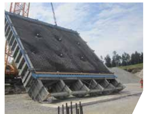
Fig. 34: Test no. 11 TECCO® G65/3 + P33, nail grid 3.5 x 3.5 m, sandy gravel 0 - 63 mm, \alpha = 53^\circ , first slides close to the surface
