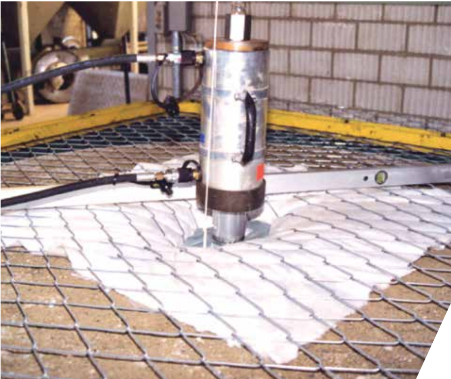
Fig. 28: Test setup to determine the bearing resistance of the mesh against puncturing in nail direction
