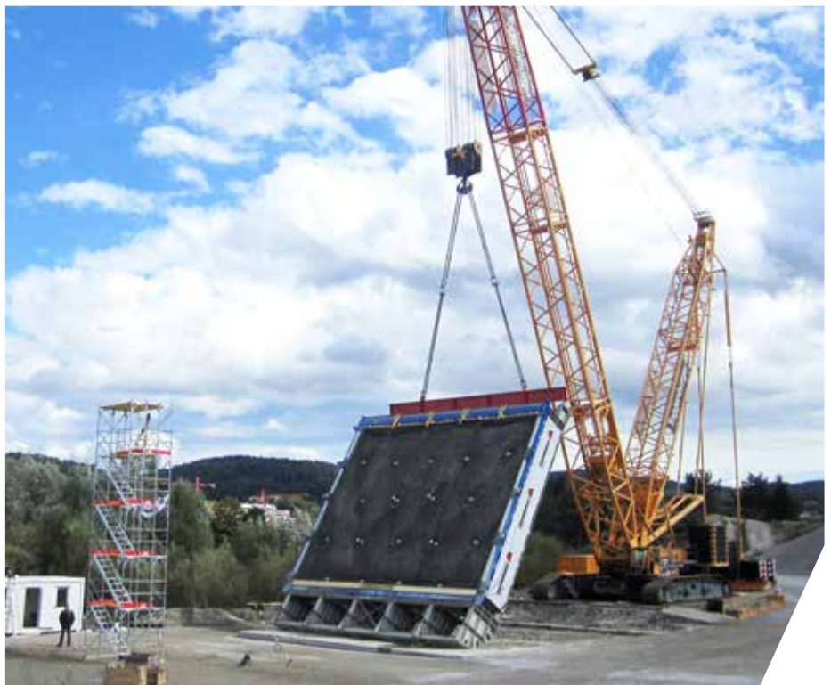
Fig. 29 (above): Test no. 13, TECCO® G65/4 + P33, after dismantling mesh cover and removing material, nail grid 3.5 x 3.5 m
