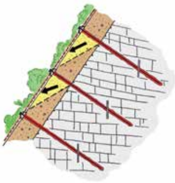
Fig. 10: Local instabilities between the individual nails
